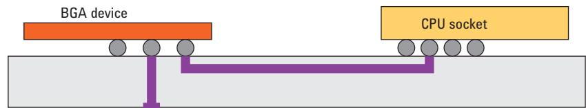
Figure 1. Hidden trace without access between BGA device ball and CPU socket ball
